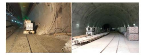
Figure 1 ACCIONA platform wagons (source ACCIONA)
