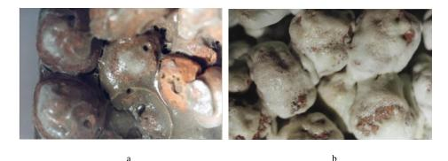
Fig. 2. Contact zone of the calcining bundle without swelling (a) and with swelling (b) of the vitreous binder.
