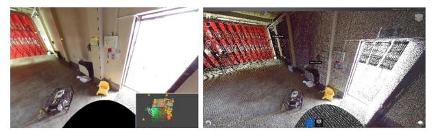
Where possible, the use of recurring strong planar surfaces in the survey environment were captured in adjacent scans to later allow the registration software to later join the individual scans into a shared coordinate system. Where this was not possible, for instance transferring the scanner around corners or through door openings, reference spheres were utilised in triplicate, for triangulation, to transfer the survey stations.
