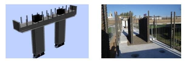
Figure 2. Interface details between the precast crosshead and the precast piers; (a) 3D view of the precast crosshead and precast piers; (b) A photo of the connection between the two components
